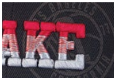
DIRECT LASER ETCHING ON CAP WITH 3D EMBROIDERY
